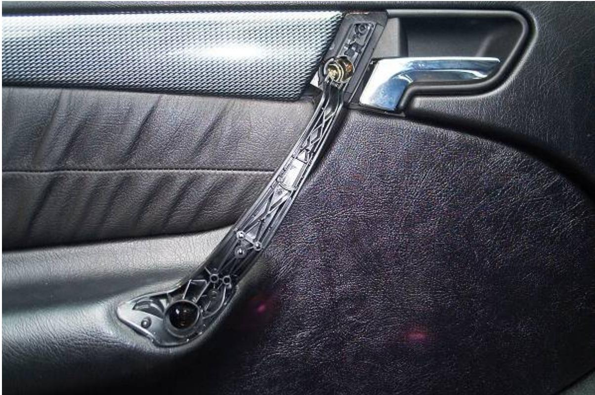
take the screw off the plastic piece around the lock end of the door:
