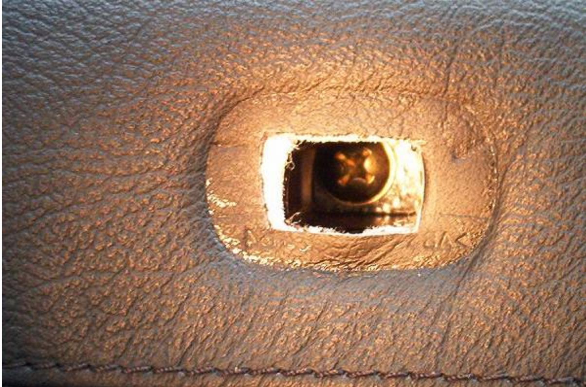
Pull the outer part of the grab handle until it comes off, it's not easy but you can slip a screwdriver in the gap at the top to ease it out, be careful as the panel is very easy to damage.
