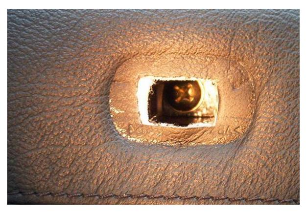
Pull the outer part of the grab handle until it comes off, it's not easy but you can slip a screwdriver in the gap at the top to ease it out, be careful as the panel is very easy to damage.
